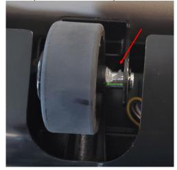
6. Spin the wheel while sliding it back and forth on the axle. Repeat 5 times.
